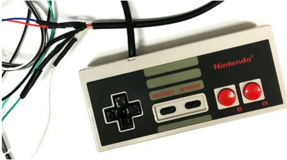
Figure 6. Original NES Controller with Internal Wires Exposed
